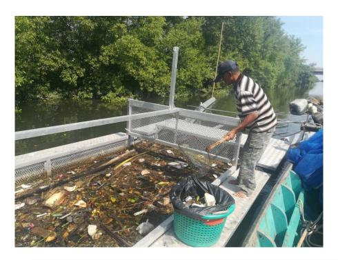
Pictured above: The special river plastic capture trap, newly installed in the waterway of Khodpor public park in Rayong, Thailand in operation. The newly installed device intercepts plastic debris before it enters the ocean.
